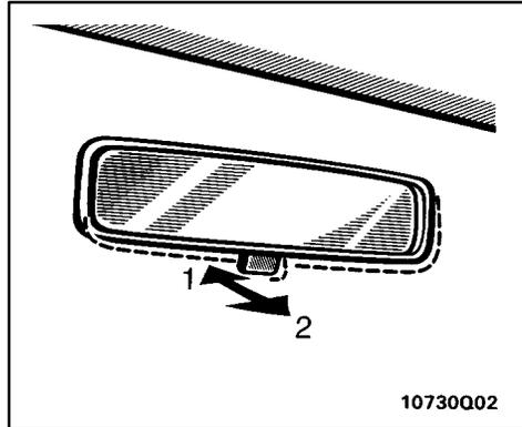
To reduce glare from the headlights of the vehicle behind you during night driving, operate the lever on the lower edge of the mirror.
