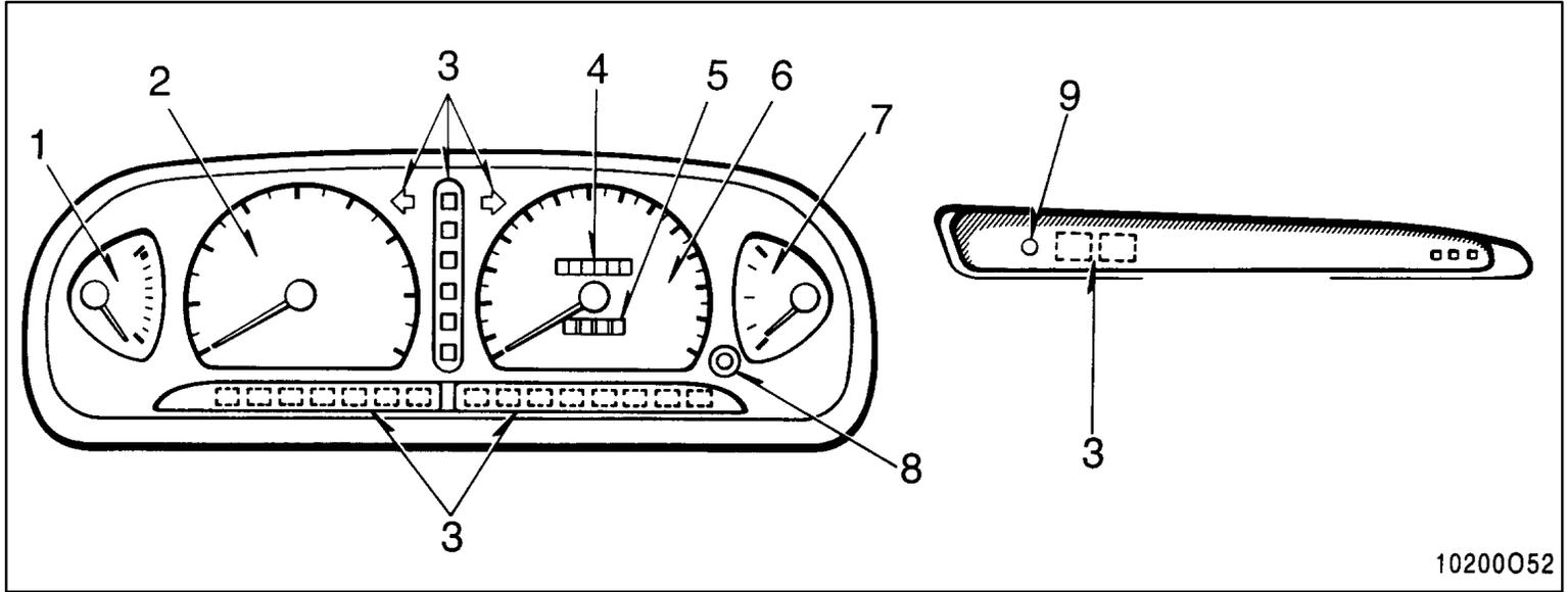
1. Engine coolant temperature gauge
