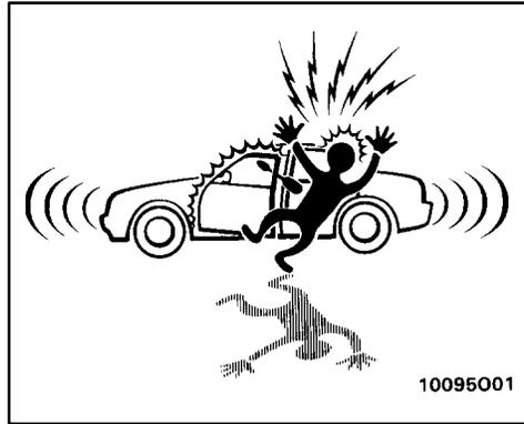
To deter the vehicle theft, the system is designed to give an alarm and keep the engine from being started if any of the doors, trunk or hood is forcibly unlocked or the battery terminal is disconnected and then reconnected when the vehicle is locked.
