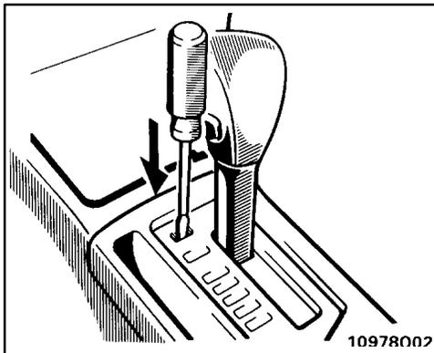
3. Insert your finger into the hole to push down the shift lock override button. You can shift out of “P” position only while pushing the button.
