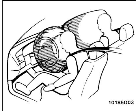
The SRS (Supplemental Restraint System) airbags are designed to provide further protection to occupants in the following seats when added to the primary protection provided by the seat belts.
