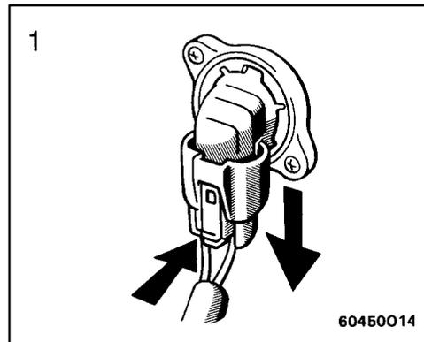
1. Unplug the connector while depressing the lock release
